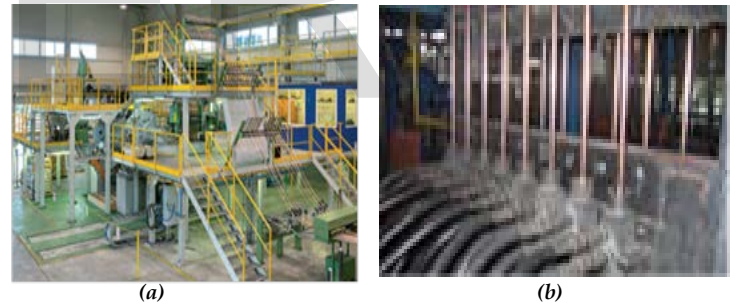
Fig. (1) UPCAST machinery (a) and Crystallizers (b).
